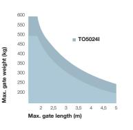
The shape, the height of the gate and the weather conditions can considerably reduce the values shown in the graph to the side. Use in windy areas 230 Vac models.
